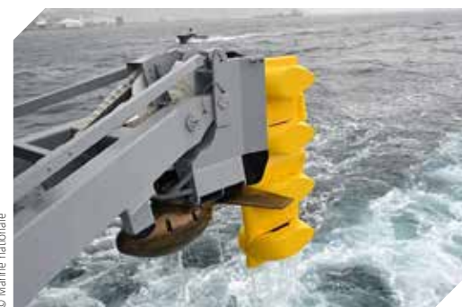
A Thales Captas sonar on board a French FREMM multimissions frigate.
